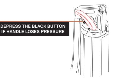
NOTE: If the handle loses pressure during pumping, depress the black pressure relief button which is located under the red lowering lever. This will allow the Jack to equalize pressure and the Jack's pumping efficiency will return to normal.
